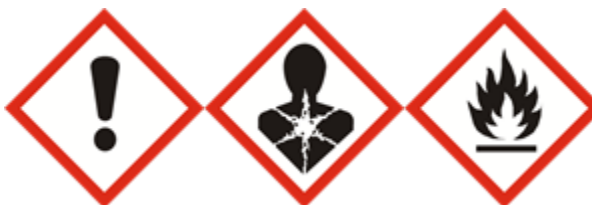
1. Exclamation mark; 2. Health hazard; 3. Flame
